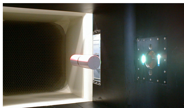
図1 磁力支持中の円柱(直径45mm円柱) (Figure 1 A magnetically suspended cylinder)
